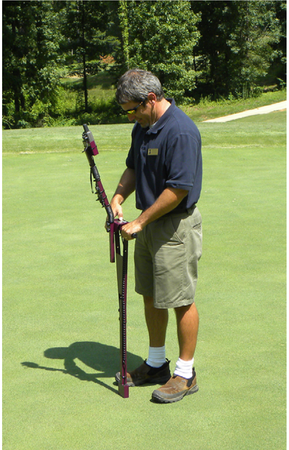
Golf Course Superintendent Randy Gatlin uses the Field Scout moisture probe on a daily basis to more precisely measure soil moisture on the putting greens at The Robert Trent Jones Trail at The Shoals.
